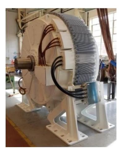
The PDD showed a significant increase in efficiency to the wind turbine, but during build of the permanent magnet generator we encountered some manufacturing challenges, including handling of high-strength magnets
